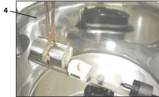
2. Place your invested flask on the appropriate flask cradle (4).
